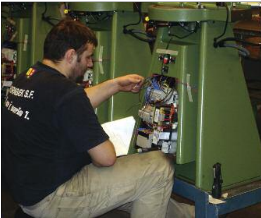
An electrician at the Morsø factory in Denmark installs the electrical components in a Morsø EH
